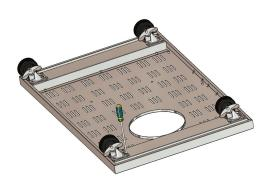
STEP-3: Attach the Right & Left Side Panel (#3 & 4) to the Bottom Panel (#2) by using 6 sets M5x12 screw with captive washer (The tank hole of Bottom Panel#2 is on the right side.)
