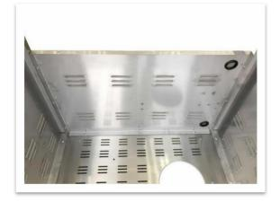
STEP-5: Attach Upper Back Panel (#6) to the Side Panels (#3 & 4) by using 4 sets M5x12 screw with captive washer, and then to use 3 sets M5x12 screw with captive washer to attach with the Bottom Back Panel (#5).
