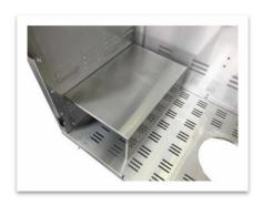
STEP-7: Attach the Tank Securing Bracket With Ring (#8) by using 2pcs plum screw, and then to use 4 sets M5x12 screw with captive washer
