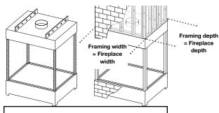
Any framing on the top of the fireplace must be noncombustible, and externally supported. Framing can be in contact with the hood, but must not use the fireplace hood to support the framing. After framing is complete, finishing materials can be extended down along the face of the unit. Do not obstruct the glass opening with finishing materials.
