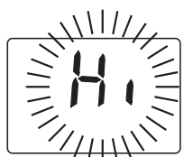
SCREEN WHILE PRESSING H/L KEY (IF PREVIOUS PRESS DISPLAYED "Lo" OR IF UNIT WAS OFF)
